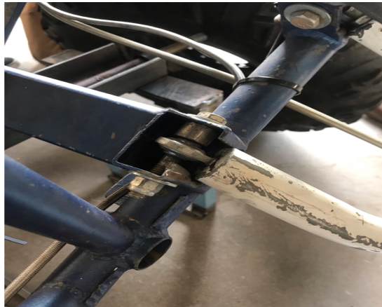
Figure 4: Bending from old heim joints
